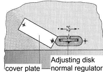
3. Make only small adjustments at any one time and pause (approx. 45 min) so that the effect of the adjustment can be noted on the digital display before further adjustments are made.
