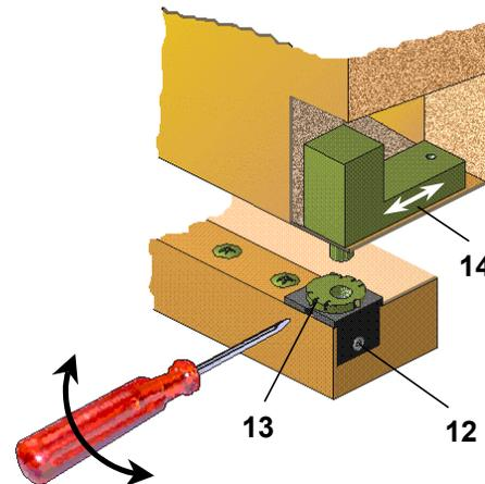
The locking plate can also be readjusted in the direction of the arrow after releasing the screw No.15.
