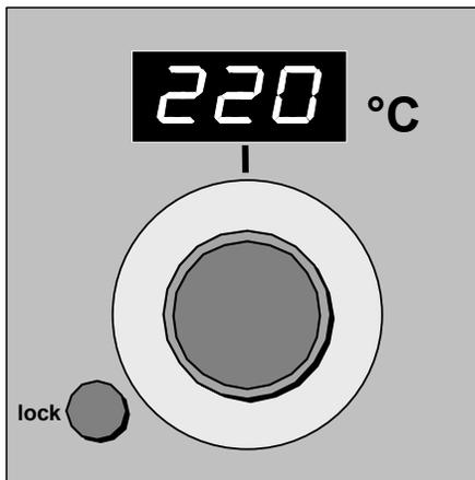
The controller is operated with the aid of the rotary knob.
